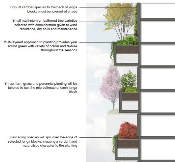
6.19 Green façades - Typical section of NE corner
